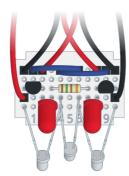
Adjust the distance between the side sensors to the width of the line. Experiment with the tilt of the sensors so that varikabi comes to a stop at the end of the line.
