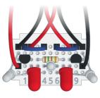
If you place varikabi some distance away from the light, it quickly moves towards the light. For varikabi to continue turning back towards the light, the tilt of the sensors has to be well adjusted.
