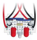
The more you point the middle sensor upwards, the closer varikabi will come the light above it. If you hold your hand between the light and varikabi, it tries to move back into the light.
