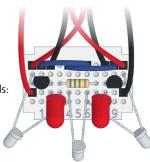
Adjust the distance of the side sensors to the size of the object. Experiment with the tilt of the sensors so that both following and stopping work well.
