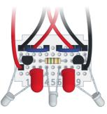
The more you point the side sensors downwards, the closer varikabi will approach obstacles. The middle sensor must be directed slightly above the obstacles.
