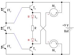
The two LEDs are arranged in series with the resistor between the transistors. Therefore, they can only light up together. In acceleration mode, they light up whenever both transistors are fully switched through.
