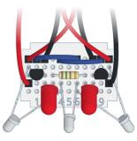
Adjust the tilt of the side sensors so that varikabi always turns in time at the edge. Adjust the tilt angle of the middle sensor so that varikabi stops at bright surfaces.
